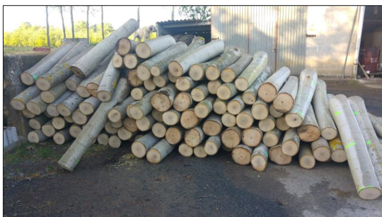
Picture 34 – Boule, typical ► air-drying system for big natural walnuts (photo Santonja)
