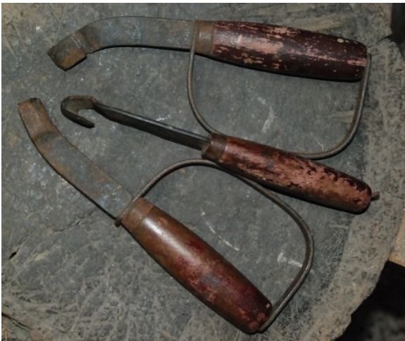
Figure 6 - Bark carving tools (scrapers).
