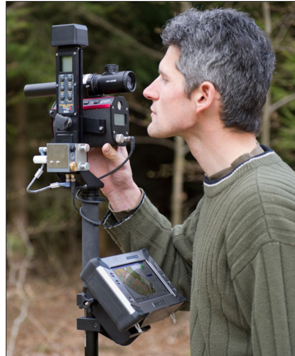
Figure 2 - FieldMap data collector (Source: http://www.fieldmap.cz/ )
